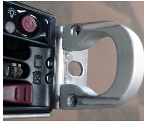
Fig. 3 - Grooves in right U-shaped handle
